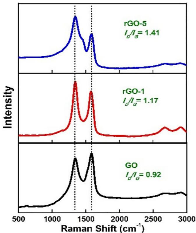
Fig. 2. Raman spectra of GO and rGO coated cotton fabric.
