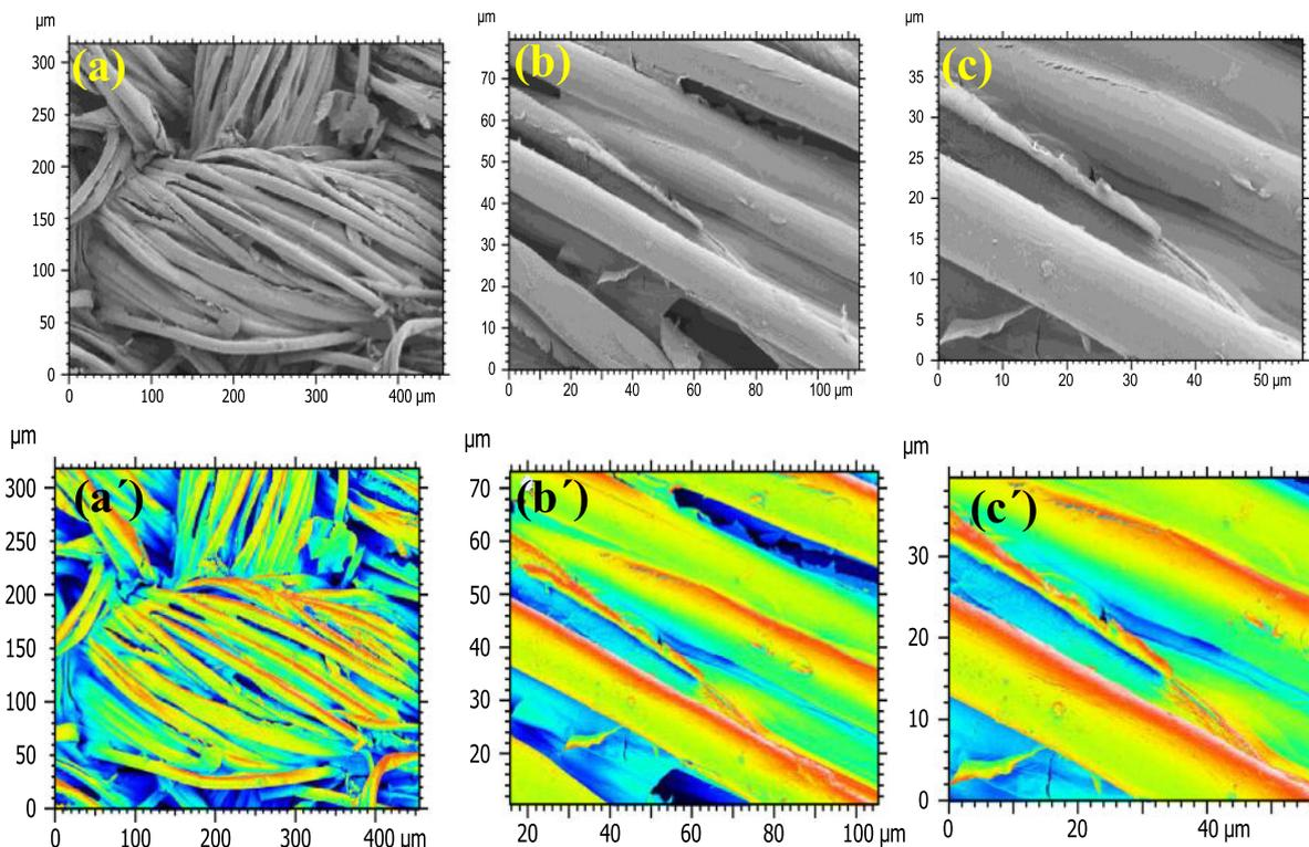
Fig. 3. (a), (b) and (c) FESEM micrographs of rGO dyed cotton fabric at different magnification and (a'), (b') and (c') colour rendering image of respective SEM images.
