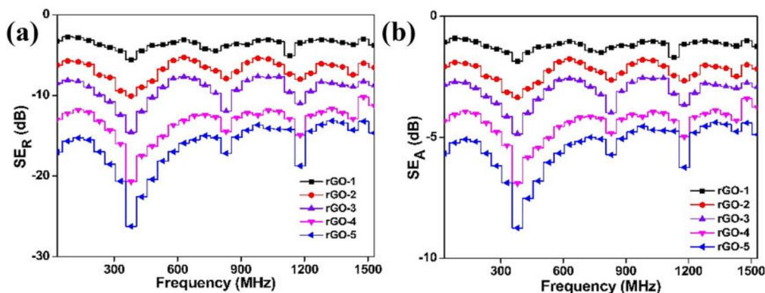
Fig. 5. EMI Shielding reflection & absorption of rGO dyed cotton fabric (a)  $SE_R$  and (b)  $SE_A$ .
