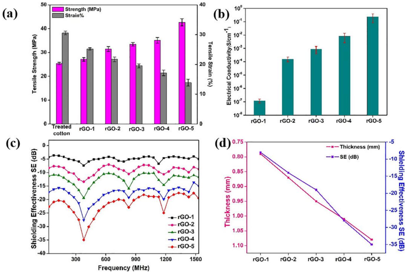
Fig. 4. (a) Tensile strength and strain%, (b) Electrical conductivity, (c) EMI Shielding effectiveness of rGO dyed cotton fabric, (d) Thickness on maximum shielding effectiveness.
