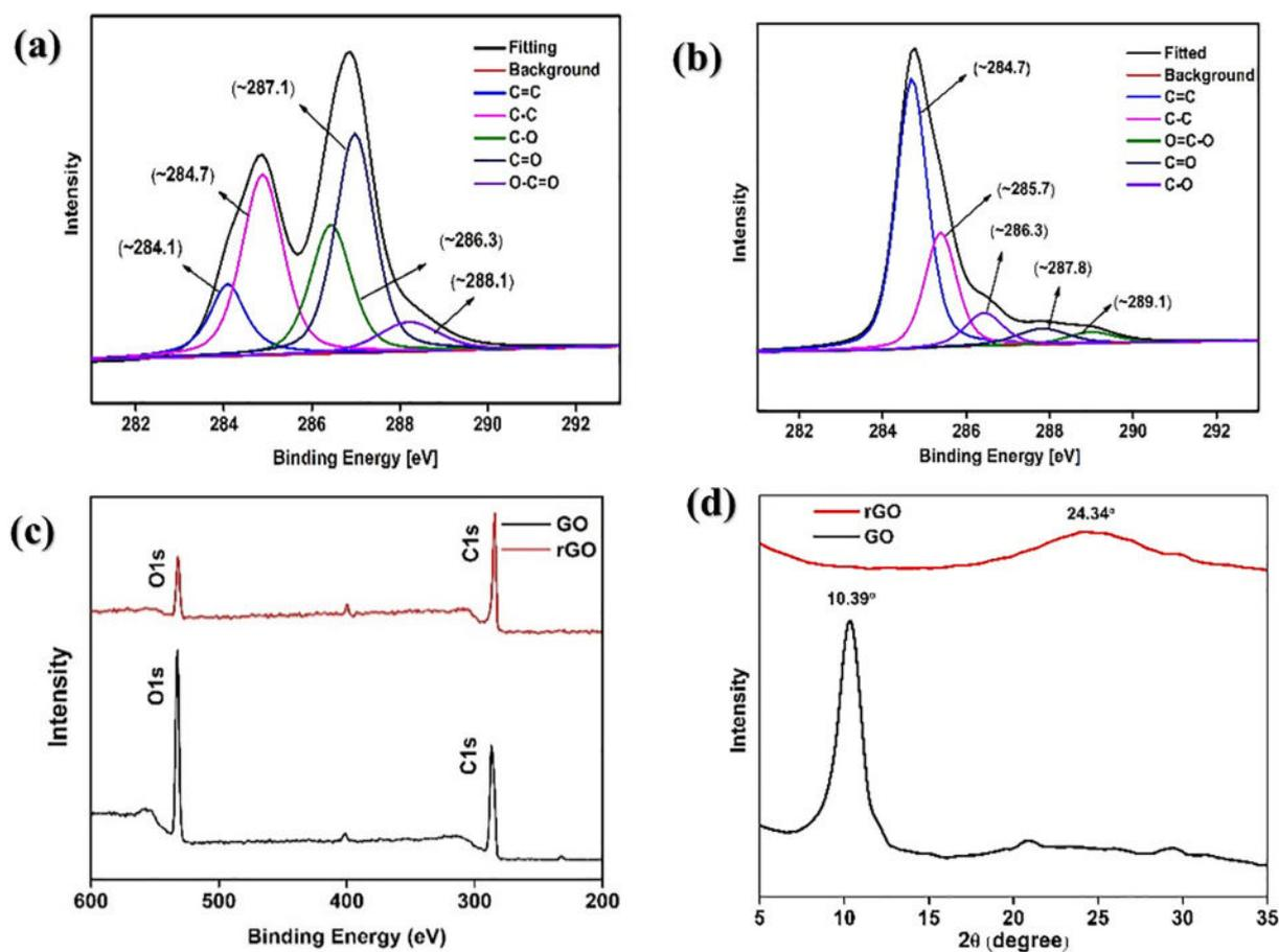
Fig. 1. XPS Analysis of GO and rGO (a) O1s, (b) C1s, (c) Survey peaks, (d) XRD analysis of GO and rGO.
