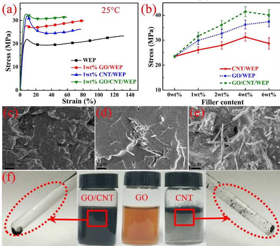
**Fig. 4.** (a) and (b) Mechanical properties of the composites; SEM images of (c) 6wt% GO/WEP composites, (d) 6wt% CNT/WEP composites and (e) 6wt% GO/CNT/WEP composites; (f) Photographs and dipping test show the dispersion of GO, CNT, GO/CNT in distilled water after 3 days.
