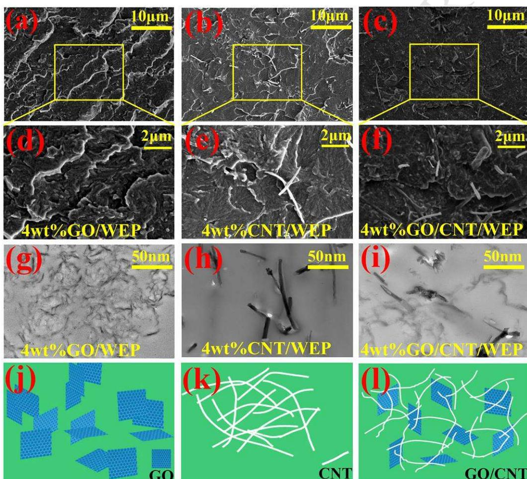
**Fig. 2.** SEM images of (a, d) 4wt% GO/WEP composites, (b, e) 4wt% CNT/WEP composites and (c, f) 4wt% GO/CNT/WEP composites, respectively; TEM images of (g) 4wt% GO/WEP composites, (h) 4wt% CNT/WEP composites and (i) 4wt% GO/CNT/WEP composites, respectively; Schematic of (j) 4wt% GO/WEP composites, (k) 4wt% CNT/WEP composites and (l) 4wt% GO/CNT/WEP composites, respectively.
