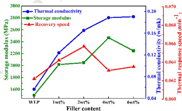
**Fig. 7.** Relationship of storage modulus, thermal conductivity and thermal response speeds of the GO/CNT/WEP composites.
