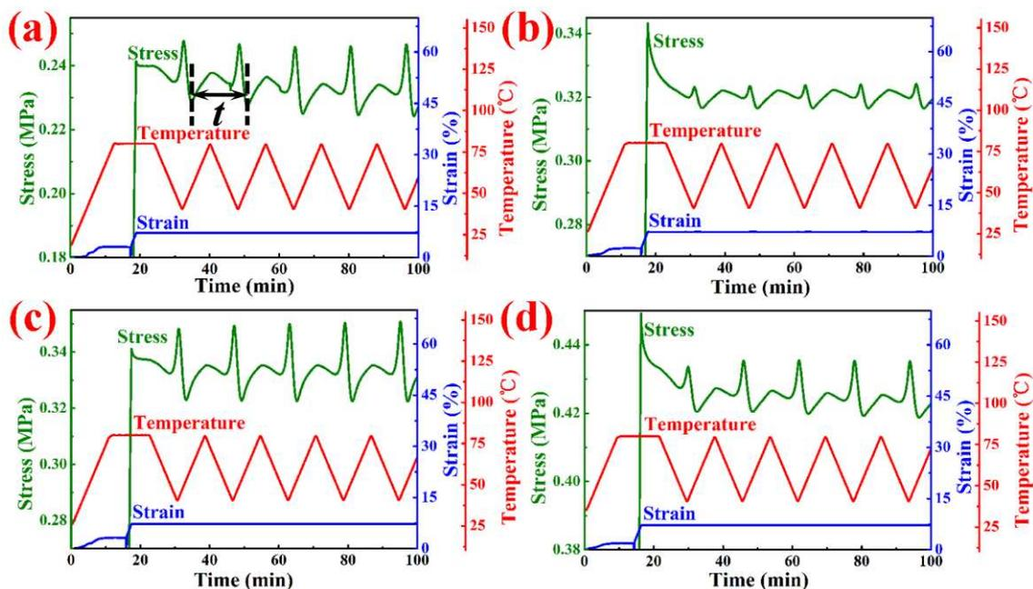
**Fig. 6.** Thermal response speeds of WEP and its composites: (a) WEP; (b) 1wt% CNT/WEP composites; (c) 1wt% GO/WEP composites; and (d) 1wt% GO/CNT/WEP composites.
