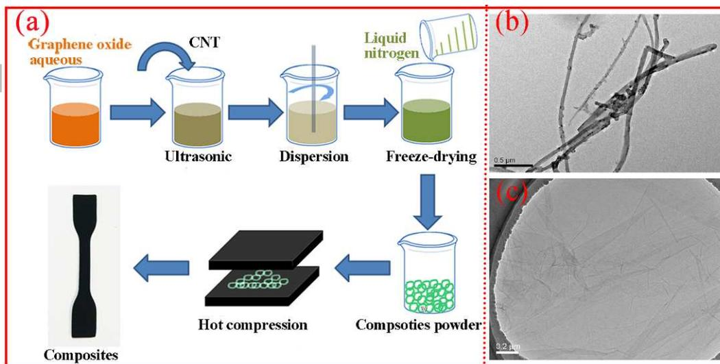
**Fig. 1.** (a) Preparation procedures of composites; TEM images of (b) CNT and (c) GO.
