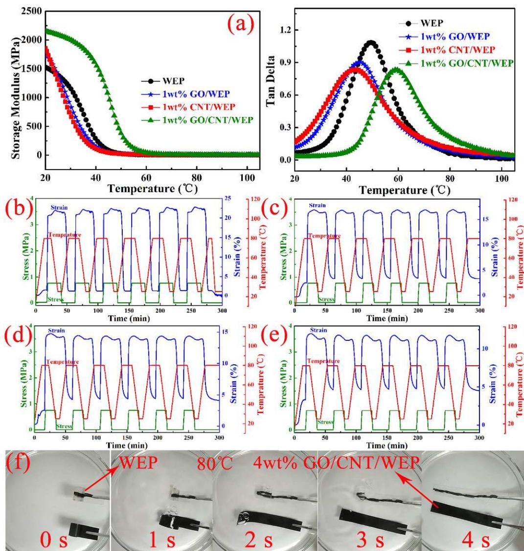
**Fig. 5.** (a) Storage modulus and Tan Delta of the composites; Thermal mechanical cycle of (b) WEP, (c) 4wt% GO/WEP composites, (d) 4wt% CNT/WEP composites and (e) 4wt% GO/CNT/WEP composites, respectively; (f) Shape recovery behavior of the samples at 80 °C.
