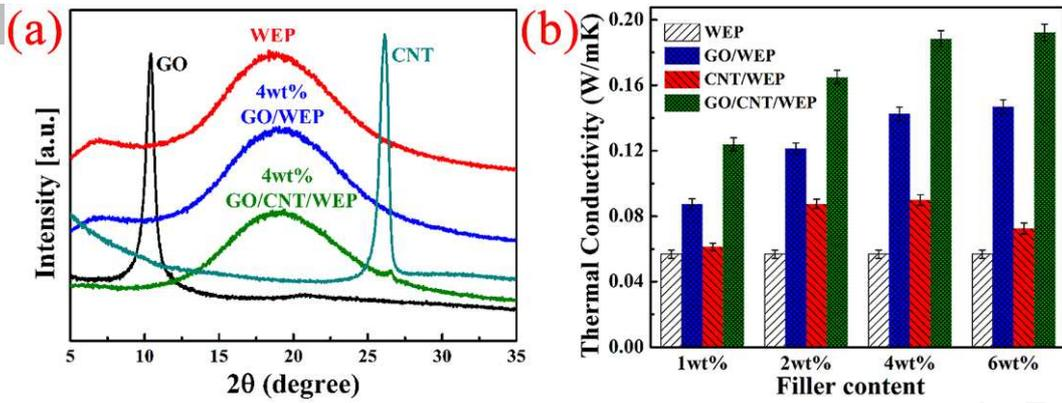
**Fig. 3.** (a) XRD spectra of GO, CNT, WEP, and its composites; (b) Thermal conductivity of the composites.
