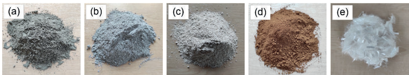
Fig. 4 Materials: (a) Portland cement, (b) silica fume, (c) stone sludge powder, (d) electric arc furnace dust, and (e) polypropylene fibers
